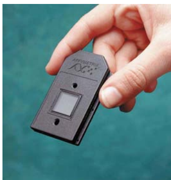
Affymetrix GeneChip® probe array. Image courtesy of Affymetrix.
